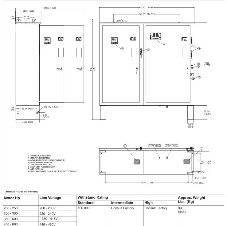
\* Coils Available: 380V-50Hz, 380V-60Hz, 415V-50Hz, 415V-60Hz
